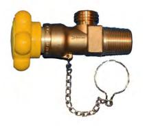
**Chlorine cylinder valve** made with O-ring sealing system and spindle thread outside gas wetted area. Valve seat and lower spindle are made of stainless steal, upper spindle is made of brass.
